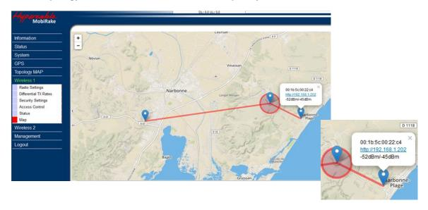
Map of the Mesh Topology – includes IP / MAC address, Frequency, RSSI and Data rate info.
